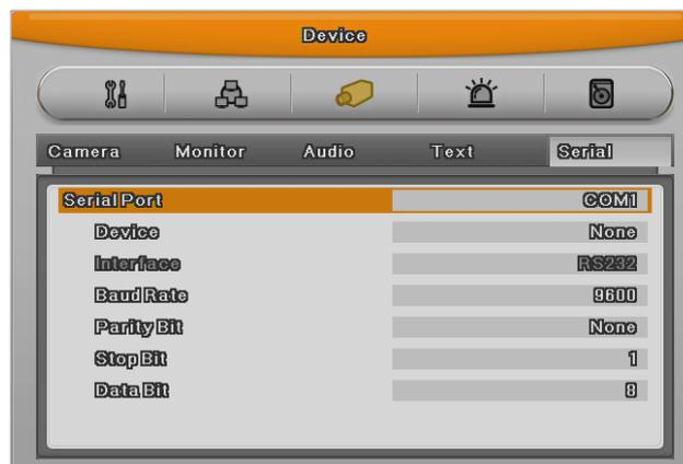
From serial setting, you can set protocol, port, baudrate, parity bit, stopbit and databit.
