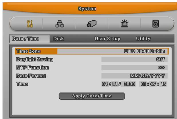
Time configuration is very important to protect the recording data. Time change on recording is not recommended. Time zone configuration value of factory default is "UTC 00:00 Dublin"
